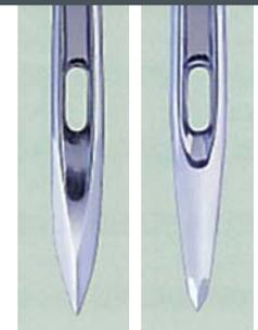
11 On the right in the photo is a SAN 5 needle with an SD point. It has a small triangular cutting tip that we use for sewing lighter gauges of polycarbonate. We like this point as we get less residue from making the hole on the backside of our sewn piece. The finished enclosure panel looks better on the backside because the cut piece of polycarbonate drops into the tray under the machine. On the left is the D/TRI point that we use for sewing heavier polycarbonates.
