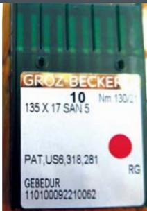
8 This is a photo of the Groz-Beckert SAN 5 needle we use most often at Hood Canvas. The figure in the upper left 135 X 17 is the only needle system that will work on our Juki LU-1508N machines. The last two digits in the upper right are the size of the needle. In this case it is 21, but we use a smaller or larger size depending on the material being sewn and thread size. To the right, below the red dot, is the point style, which, in our case, is an RG.
