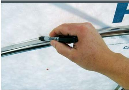
9 We mark the forward edge of the mid bow by holding a marker against the bow at an inward angle from the underside of our top. This results in an angle on the mid bow which is the same as the angle on the forward and aft bows, contributing to an even pull.
