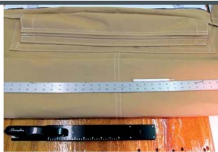
10 Ease off all mid pocket ends by 1/2-inch. Only the center of the pocket needs to be tight. Failure to do so will result in a diagonal ripple in our top. We have mentioned this in previous articles, but is worth repeating.
