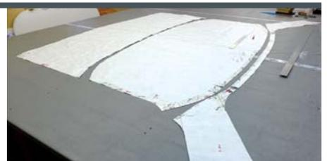
8 This is the completed pattern cut apart and ready for fabrication. The cut lines are the finish size so hem allowances will need to be added to all seams.
