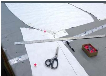
6 Back at the shop, we have started working up our pattern. This is the aft end where the top and tails meet. Notice the darts at the mid bow and the tails for proper fit. We have rounded the inside connection between the top section and the tail. This adds a touch of styling and if we were to add side curtains, this would enable the attachment zipper to round the corner.
