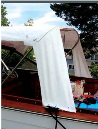
4 We added another layer of double-sided sticky tape on top of our pattern and stick on a square of pattern material to make our sport top tails. Be sure it lays in smooth and fits the contours of the frame. Now mark the cut line on the aft bow.
