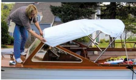
1 Deb is fitting the forward edge of our pattern first, so it is smooth between the mid bow and the windshield.
