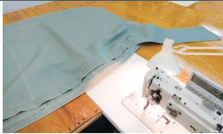
10 We have top-stitched the aft end. Be sure the aft bow pocket is out as shown in the photo. Also notice that the tail and visor are connected as one piece.
