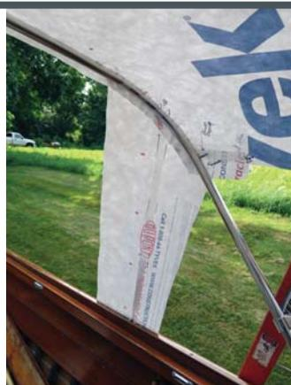
5 This is a view from the underside showing the overlap of the tail pattern pieces. Notice the strapping tape at the hold-down strap position inside the tail, so it is hidden. The strapping tape is holding the upward force of our frame preload down the center line of our frame. It is important that the strapping tape is placed at the exact spot that our strap will be when our sport top is completed for proper preload and fit.
