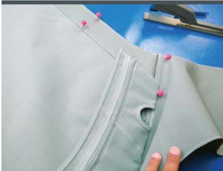
12 This is the end of the aft pocket, cut up to allow a zipper to pass. We have pinned out the side to remove any waviness prior to stapling the aft pocket down as this is important to the final fit. Notice the cutout for our hold down strap just inside the wing. This is in the exact spot that we had out strapping tape while patterning.
