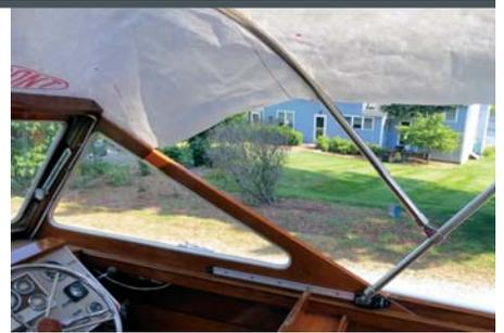
3 This is a view from the underside. Notice the marker line from when we fitted the forward section. We now have to draw another line after fitting the aft section. These lines merge near the center of the frame creating a dart of excess material to be removed in later steps.
