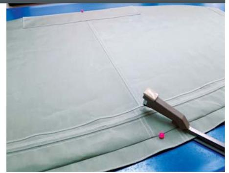
11 The bow pocket is flipped to the underside. Notice we have pinned out the center seam prior to stapling the pocket down. Failure to do this with any top will result in a non-even pull and will cause wrinkles when installed.
