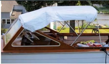
2 Now, after marking the forward edge of the bow from the underside, we release our pattern from the double-sided tape and re-stick. We want our pattern to be smooth between the mid bow and the aft bow. These steps are performed on each side of the boat after initially securing our pattern blank along the center line of the frame and windshield.
