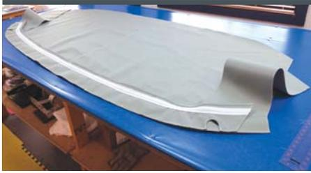
9 Here the aft end is assembled and stapled in the proper stacking order prior to stitching.
