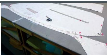
7 Here we have added a visor extension to bridge the gap between the two tails. Notice again that we have rounded the corners to facilitate a zipper for an aft angle back should the owner ever want one.
