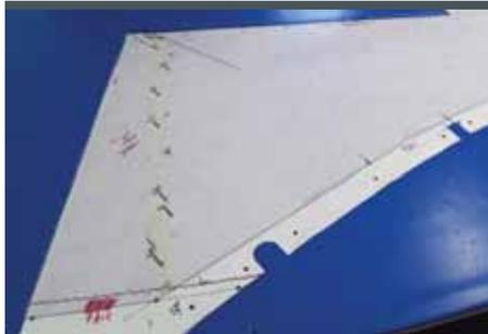
1 In this photo, we have drawn lines and punched holes in our pattern where the clear vinyl and the fabric are to be joined. Notice in the bottom left-hand corner that our joining line extends to the edge of the pattern on the right-hand side. Below this line is the second piece of fabric we will cut to overlap onto the top assembly. Our clear vinyl has been cut to these innermost lines and is laying on top of the pattern in the photo for clarification purposes.
