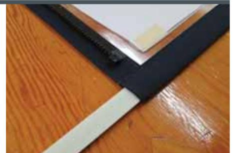
10 This photo shows detail on how the two fabric pieces overlap. At this point the pattern should match the fabricated side curtain exactly. If any of the fastener locations are askew, we will correct them using the pattern.
