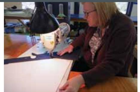
7 & 8 Deb is applying the bottom fabric piece using the same procedure. These photos show a little more detail of the seam tape applied to both sides and the folding of the outside fabric. Notice that the seam tape extends onto the fabric of the previous step. There is a finished overlap of  $\frac{3}{4}$  of an inch extending off the clear vinyl onto the fabric of the previous step to the bottom edge of the side curtain.
