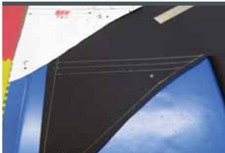
4 Using the same procedure, we have cut out the bottom section of fabric that will be attached to the clear vinyl. Once again be sure to keep the fabric in the same selvage-edge-to-selvage-edge orientation. With the bottom attachment piece we need to follow the line on the pattern to the far right past the clear vinyl to the bottom edge of the side curtain.
