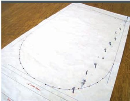
**1** This is our pattern with the smile window marked on it with a Sharpie marker. We punch holes along the length of the smile so that we can transfer the center line marks of the smile to the window vinyl underneath. We also use the pattern to transfer the center line marks to the fabric used to make the cover flap.
