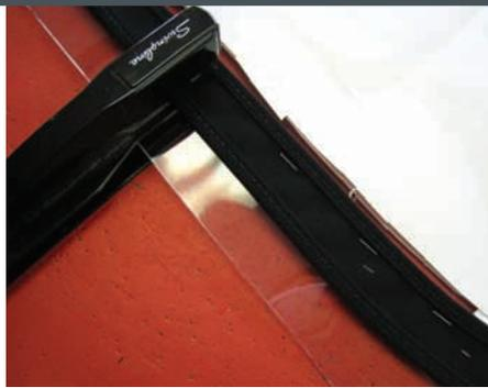
8 The cover flaps are now stapled with a long-arm stapler to the outside of the window vinyl. It must cover the zipper installed on the inside of the window vinyl. This is where the extra 2 inches at the top of each side of the cover flap is needed to account for any small adjustments in alignment.
