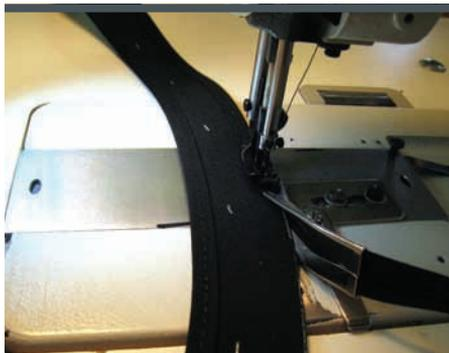
**4** We now bind the inner and outer side of each cover flap with ¾-inch binding. Keep in mind that this is a single-ply cover flap.
