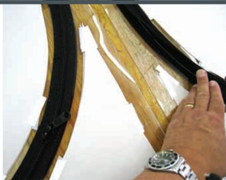
11 This is the completed smile window with cover flap installed. It is now ready for adding the top, bottom and sides. With our 1½-inch large binder, this is accomplished in short order for the sides and top.
