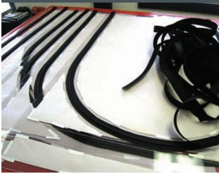
7 The stack of smile windows with zippers installed, and finished cover flaps ready to be installed.
