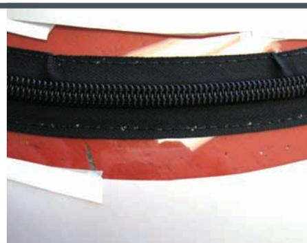
**6** A close-up of a section of the zipper with a couple of material pleats in it along the inside edge as it goes around the curve.
