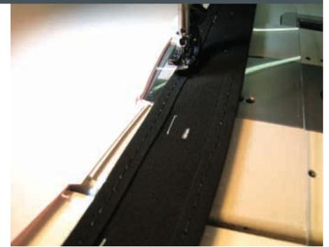
9 Starting at the top inside edge, stitch the cover flap on each smile. Stitch on the binding stitch line and remove the staples. Do not stitch the outside edge or your window will not open. In the case of a "frown" instead of a smile, stitch the cover flap on the outside edge and leave the inside edge unstitched.
