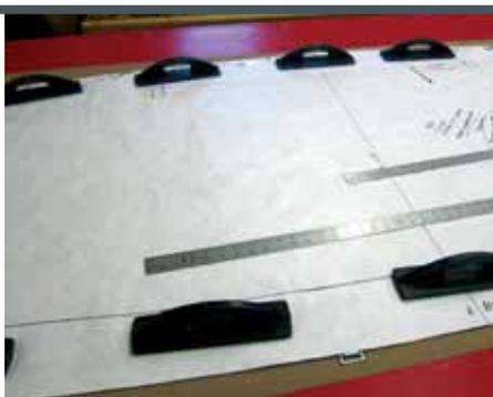
5 Here we are laying out the top aft panel. Notice that we have pinned out the seam to put it in its natural state before placing the pattern on top with weights. We use a strap adjuster buckle under the edge of the pattern to mark our 1/2-inch seam allowance.
