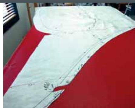
3 A close-up of one side curtain is shown here. We have punched holes where the fabric bottoms join the clear vinyl. This is done in two sections: the bottom piece and the piece that runs forward along the windshield. This facilitates fabrication in that no one joining piece is wider than the width of the fabric.
