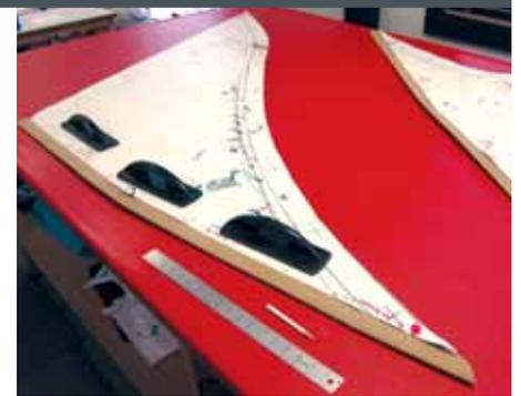
8 In this photo we have the side curtain patterns on top of the side curtains in order to transfer the hash marks for proper side curtain alignment with the Navy top. First we stitch the zips onto the Navy top and then we transfer the hash marks to the bottom of the zipper from the hash marks on the Navy top. Finally, we remove the bottom half of the zips and align and stitch them to the hash marks on the top of the side curtains.
