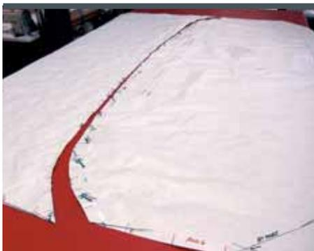
4 In this photo we have cut the side curtains off the pattern and cut the top mid seam apart on the pattern along the marking on the underside for the secondary bow. We transferred this line from the underside to the outside by using a rolling pounce wheel to make perforations. Notice that there are hash marks for seam and zipper alignment where the pattern pieces are separated.
