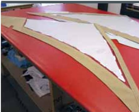
9 These are the almost-complete side curtains. We have used our large binder to finish the top edges. We need to add the aft sleeves that hold 1-inch flat battens to stiffen the aft edge from flapping while underway. We also need to bind the bottom edge, but first let's go over the fabrication of the aft sleeve.
