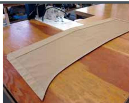
6 This photo shows the forward section of the Navy top with the sides folded in and the forward reinforcement in place, stapled and ready for stitching. We will add rubber spray welt and binding to the forward edge where the snaps will go.
