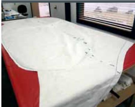
1 Here is the rough pattern as we removed it from the frame in the last article. Notice that it does not lay flat on the table as there was extra material removed from the forward section.
