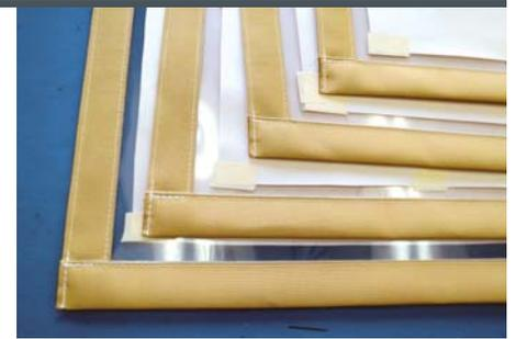
9 The completed enclosure pieces. Here we have added a stitch along the top edge of each panel and heated the tops of the vertical strips so they will not fray.
