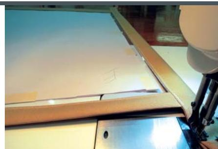
6 We like to start our binding off the enclosure and run onto the enclosure and off again as in the photo. With the inch of free space, we can back tack with no problem. By running strips through the binder by themselves we make up all of our roll-up straps. Just add a stitch to the other side and cut to length. Notice that we add the top binding strip first, then overlap the vertical binding strips.
