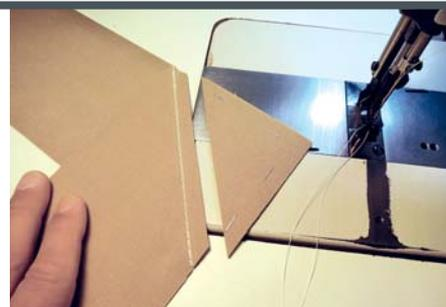
3 In this photo, we have stitched along this line and cut the corner off to approximately half an inch from the line.
