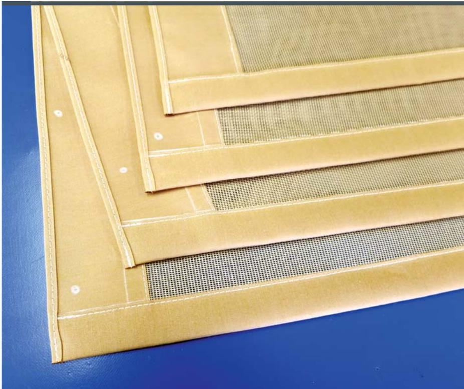
10 The identical screen replacement panels with binding added to the bottom edge. We install the zippers on our screen panels so they exactly match our clear panels. In this way our customers can mix and match clear and screen panels in whatever combination suits them. Our customers love this feature.
