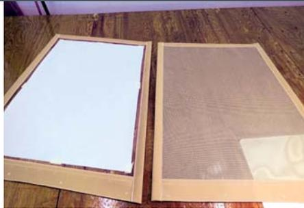
8 While we are at it, we made up some replacement screen panels. We find it is faster using our binder to make up identical interchangeable panels. Adding detail by combining clear and screens on one panel takes up too much time and adds weight. In the photo, we have trimmed the vertical strips even with the top and bottom of our enclosure pieces.
