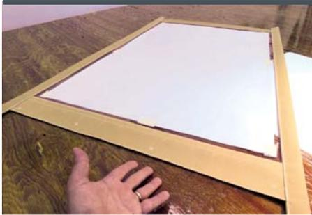
7 In this photo, the vertical strips are installed. It takes us about an hour and a half to install all the tops and sides on a 10-piece enclosure.
