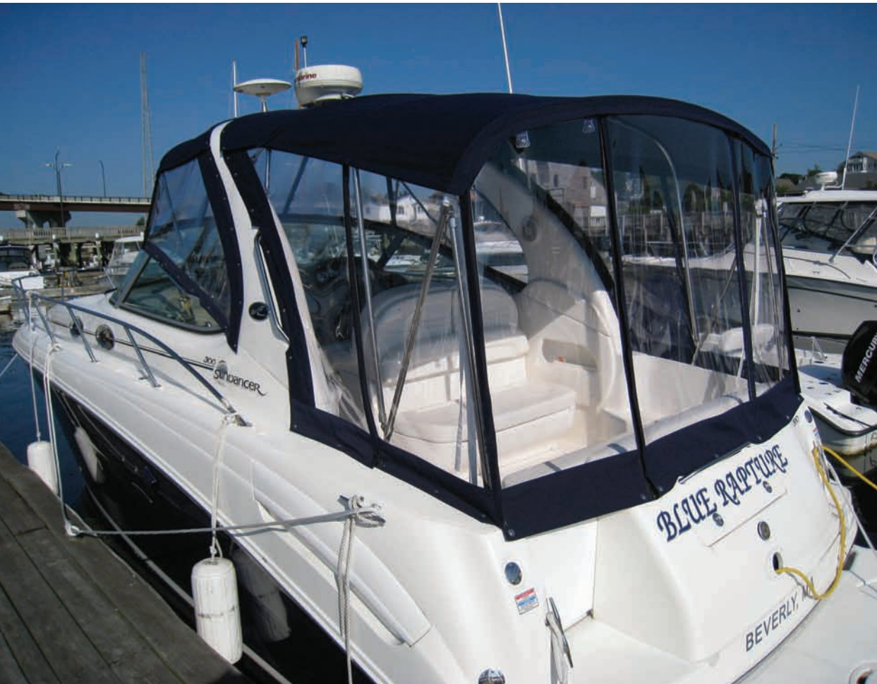
A Hood Raised Enclosure with camper. Notice the location of the aft corner division on the visor.
