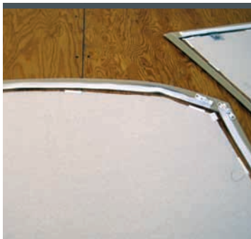
13 The panel with its zippers installed. The top zipper faces outward to hide it.
